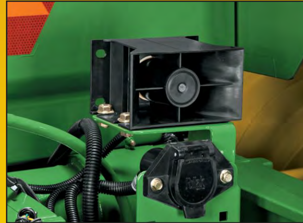
Transmission Back-Up Alarm. Sounds a loud warning when you put the transmission in reverse. No. RE224298.
